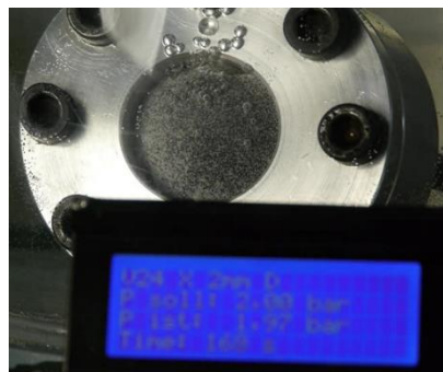
Test set-up for measuring air tightness
