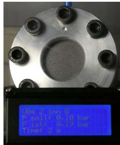
Test set-up for measuring burst pressure
