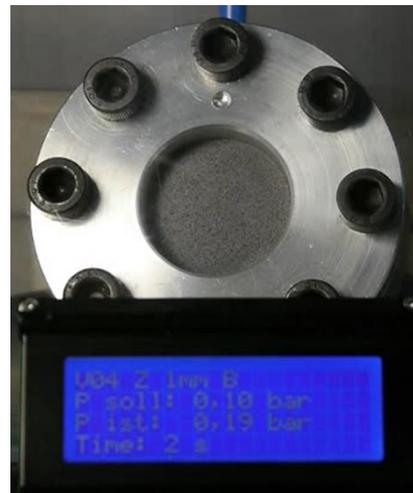
*Test set-up for measuring burst pressure*
