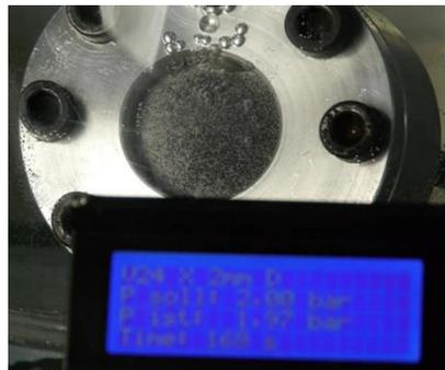
*Test set-up for measuring air tightness*
